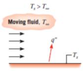
In this case the proportionality exist between temperature difference  $(T_s - T_{\infty})$  and the heat flux q" as
