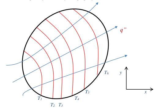
If  $T_1 > T_2 > T_3 > T_4 > T_5 > T_6$ , heat flow in unit area (heat flux) perpendicular to the isotherms in a proportional manner as
