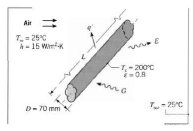
The surface emissive power may be evaluated from Equation 1.5, while the irradiation corresponds to  $G = \sigma T_{sur}^4$ . Hence
