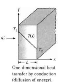
$$q''_{x} = -k \frac{T_{2} - T_{1}}{L}$$
