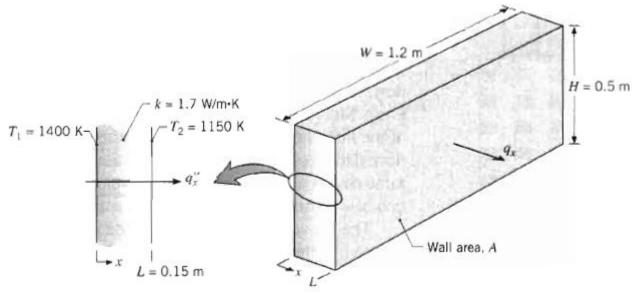
For the steady state condition temperature profile is linear,
