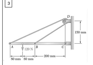
Find the support reactions and the force of the cable ADB of the given structural system.
