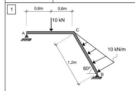
Find the support reactions of the given structural system.
