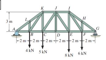
Determine the force in members JK, CJ, and CD of the truss system. Specify whether the members are in tension or compression.
