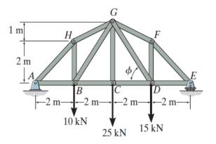
Determine the force in members GF, GD, and CD of the truss system. Specify whether the members are in tension or compression.
