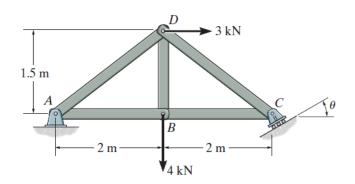
Determine the force in each member of the truss system and specify whether the members are in tension or compression.  $\theta = 30^{\circ}$ .
