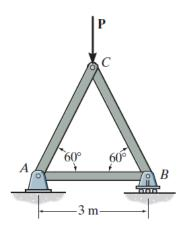
Determine the maximum value of P that can be applied to the truss system so that no member is subjected to a tensile force exceeding 2 kN or a compressive force exceeding 1.5 kN.
