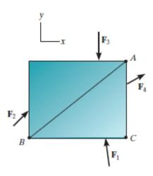
When a body is subjected to a system of coplanar forces, which all lie in the xy plane, the forces can be resolved into their x and y components. Consequently, the conditions for equilibrium in two dimensions are
