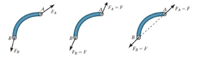
For any two-force member to be in equilibrium, the two forces acting on the member must have the same magnitude, act in opposite directions, and have the same line of action, directed along the line joining the two points where these
