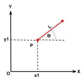
To define/constraint the position of a line L or a planar rigid body, its distance from the origin in x and y-axis and the angle from x-axis is required. Therefore, the line L or a rigid body has three DOFs in 2D space. The position and orientation of a rigid-body in a plane is defined by two components of translation and one component of rotation, which means that it has three DOFs.
