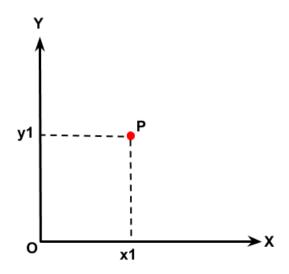
To define/constraint the position of a point P in a plane, only its distance from the origin in x and y-axis is required. Therefore, the point P has two DOFs in a plane.
