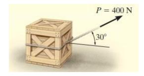
The 50-kg crate shown rests on a horizontal surface for which the coefficient of kinetic friction is  $\mu k$ =0.3 If the crate is subjected to a 400-N towing force as shown, determine the velocity of the crate in 3 s starting from rest.
