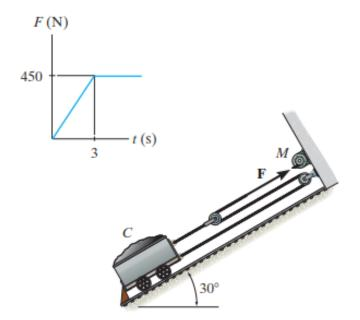
If the force of the motor M on the cable is shown in the graph, determine the velocity of the cart when t = 3 s. The load and cart have a mass of 200 kg and the car starts from rest.
