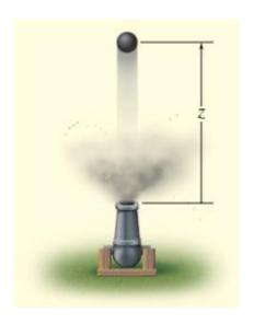
A 10-kg projectile is fired vertically upward from the ground, with an initial velocity of 50 m/s. Determine the maximum height to which it will travel if (a) atmospheric resistance is neglected; and (b) atmospheric resistance is measured as
