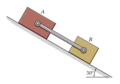
If blocks A and B of mass 10 kg and 6 kg, respectively, are placed on the inclined plane and released, determine the force developed in the link. The coefficients of kinetic friction between the blocks and the inclined plane are  $\mu_A = 0.1$  and  $\mu_B = 0.3$ . Neglect the mass of the link.
