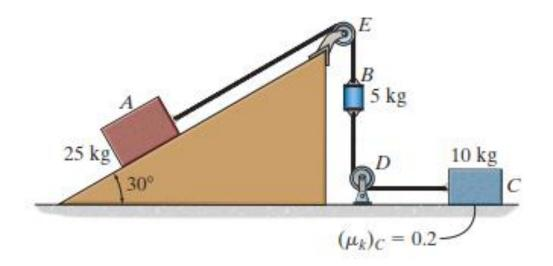
Determine the acceleration of the system and the tension in each cable. The inclined plane is smooth, and the coefficient of kinetic friction between the horizontal surface and block C is  $(\mu_k)_C = 0.2$ .
