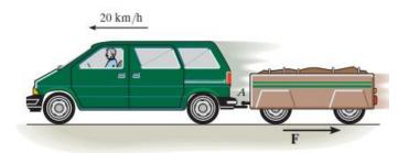
The van is traveling at 20 km/h when the coupling of the trailer at A fails. If the trailer has a mass of 250 kg and coasts 45 m before coming to rest, determine the constant horizontal force F created by rolling friction which causes the trailer to stop.
