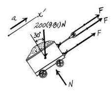
**Equations of Motion:** For  $0 \le t < 3$  s,  $F = \frac{450}{3}t = (150t)$  N. By referring to Fig. we can write
