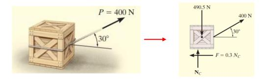
**Free-Body Diagram.** The weight of the crate is W = mg = $50 \text{ kg} (9.81 \text{ m/s}^2) = 490.5 \text{ N}$ . As shown in Fig. 13–6b, the frictional force has a magnitude  $F = \mu_k N_C$  and acts to the left, since it opposes the motion of the crate. The acceleration a is assumed to act horizontally, in the positive x direction. There are two unknowns, namely  $N_C$  and a.
